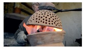
**Fig. 6.** Soldering of the Goblet copy with the analogue of Kvatskhela muffle.
